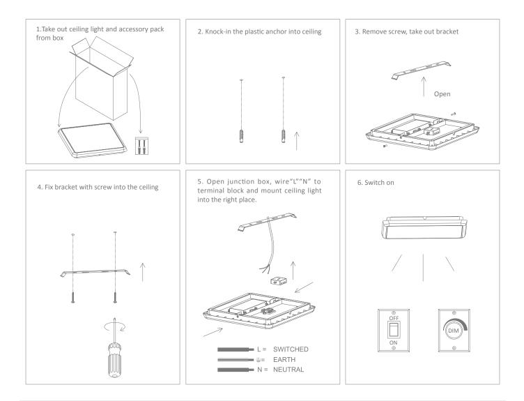
**Note:** -The lamp must be installed by professional electrician -Ensure the power supply is switched off before fitting this product -Do not touch the lamp when in use -Keep away from hot steam and corrosive gas
