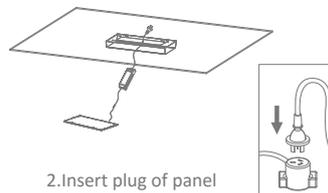
2. Insert plug of panel into mains socket.
