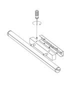
3. Knock-in the plastic anchor | 4. Remove the link pressing clip, into the wall. Fix bracket with screw into the wall
