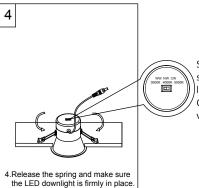
Select the colour preference by sliding the dip switch on rear of down light. (3000K, 4000K, 5000K)
