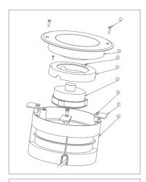
1. Drill a hole of Ø206mm in the ground, insert housing (8) "Note: Orange holders (7) must be parallel to the ground, to guarantee alignment, the use of silicon is required around the housing (8) to hold it in position"
