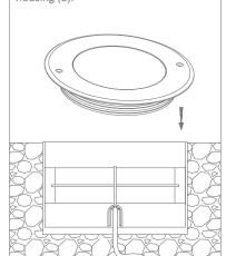
5. Fasten luminiare (2) to housing (8), using the screws (1) provided.
