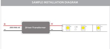
Must be used with a suitable 24v DC LED Driver
