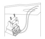
Step 3 Connect the downlight with driver, hold back the spring clip then push the downlight into the hole.
