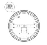
5. Remove the driver cover and line pressing clip, connect the wires correspondingly.
