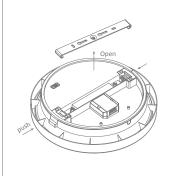
3. Knock-in the plastic anchor into ceiling. Fix bracket with screw into the ceiling.
