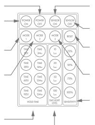
Sensor ON Button enters the last saved parameter state to be commanded.
