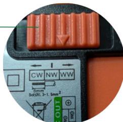
LED Driver Tri-colour selector switch (CW/NW/WW)
